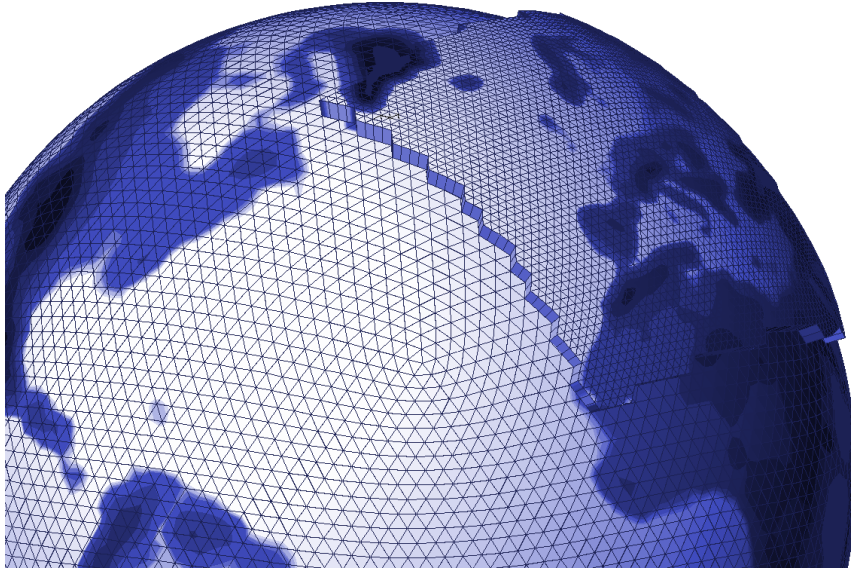
Figure 3.6.: Basic example of a multi-grid setup, consisting of a global ICON domain and a child domain over Europe with half grid spacing. Closely resembles configuration that is used operationally at DWD for deterministic forecasts with a horizontal grid spacing of 13 km globally and 6.5 km in the child domain.
